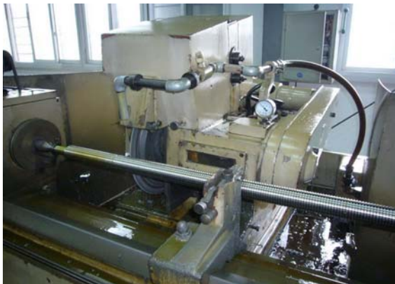
Thread grinding of Screw Shaft
